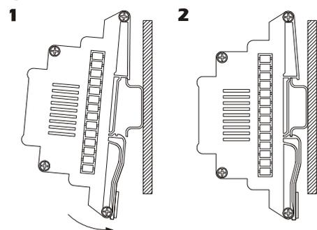
To remove C-PRO EXP MICRO, provide oneself with a screwdriver and operate as shown in the following drawing.
