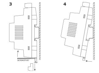
To install the device again press down the clip before
