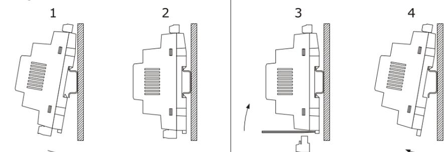
To remove the devices remove possible extractable screw terminal blocks plugged at the bottom first, then operate on the DIN rail clips with a screwdriver as shown in the following drawing.
