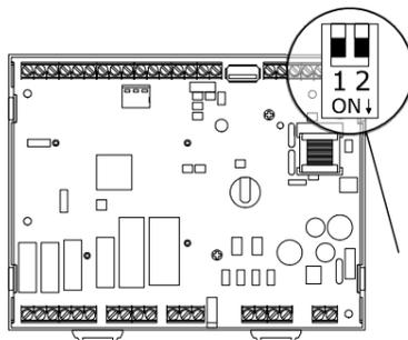
The RS-485 MODBUS network can be polarised using the UNI-PRO 3 development environment.
